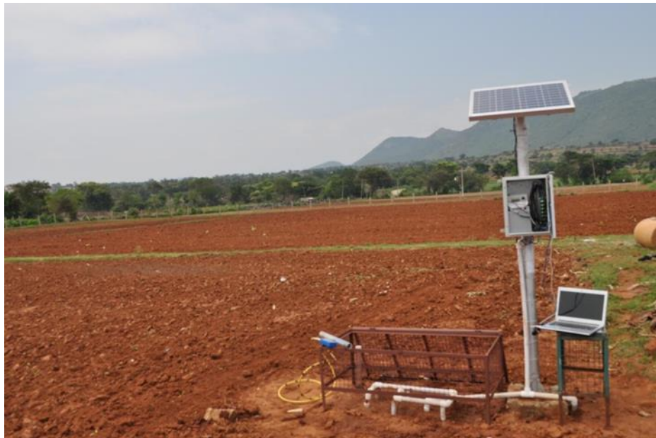
Figure 2-6: Field Assembly of HYDRA Probe Soil Moisture Sensor
