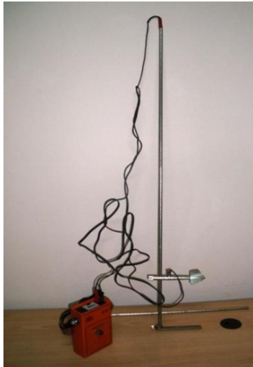
Figure 2-12: A Typical Current Meter Assembly
