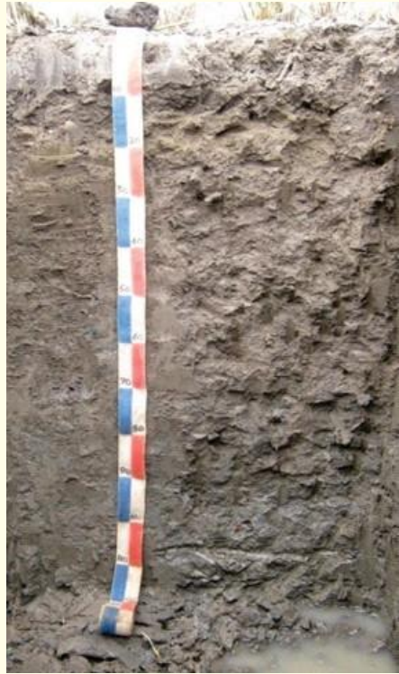
Fig.5.11 Poorly drained soils, gleyed upto the surface layer, Chikkarasinakere series, Mandya district
