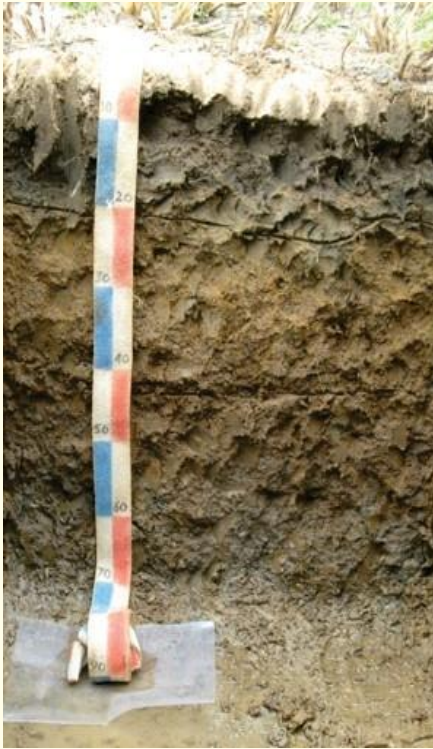
Fig.5.10 Somewhat poorly drained soils, mottles in the upper B and gleyed in the lower B horizon, Mandya district
