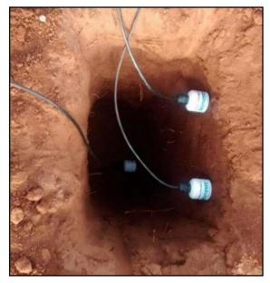
Schematic of HYDRA Probe Soil Moisture Sensor
