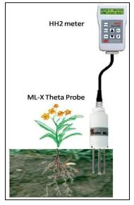
Theta probe and HH2 meter (Delta T Devices)
