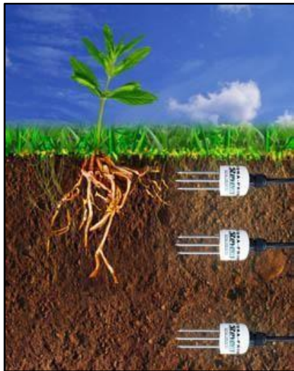
Schematic of HYDRA Probe Soil Moisture Sensor
